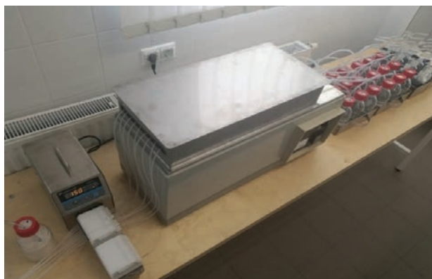
Figure 3: Measurement of the biodegradability of bioplastics using respirometry and in bioreactors at Profikomp Inc.
