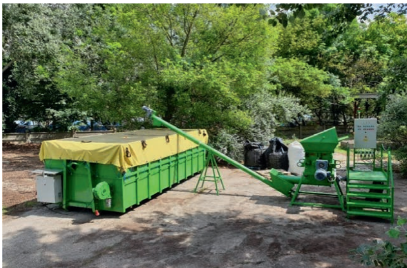
Figure 6: On-site composting of food-contaminated tableware at Sziget Festival in 2019 using ProfiKomp® technology.
