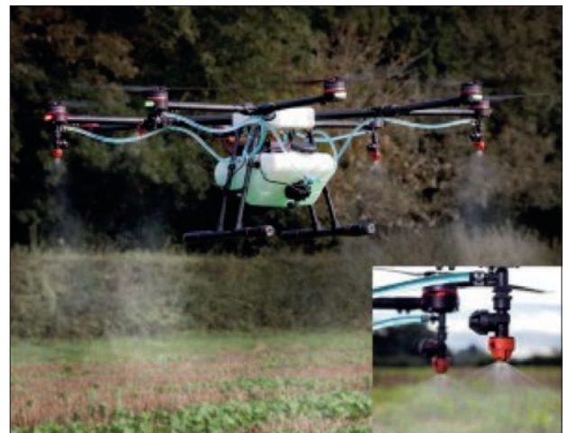
Figure 1: Drones with precision sprayers (insert) apply agrochemicals only where they are needed (Source: Anthony 2017)
