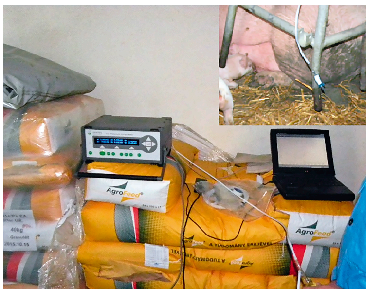
Figure 2: Measurement of the gas content of the barn air (Source: NARIC MGI)
