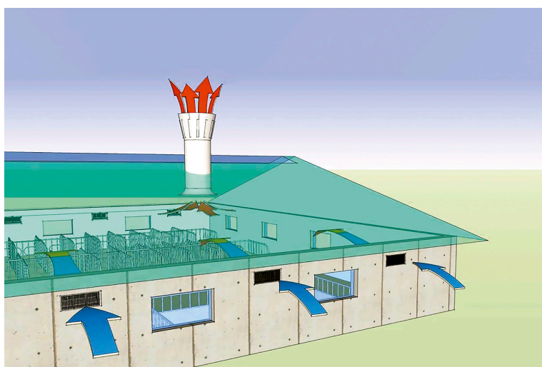
Figure 3: In case of outliers during gas measurement, the ventilation system is automatically activated (Source: Okosfarm.hu)
